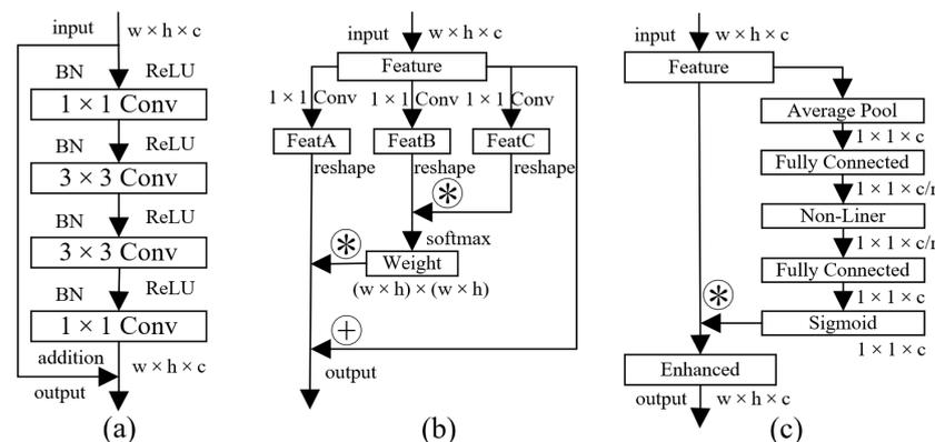
Figure 4. Details of the related blocks. (a) The residual block (RB). (b) The spatial attention block (SA). (c) The channel attention block (CA).
