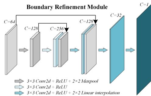
**Figure 7.** Detail of lightweight road boundary refinement block.
