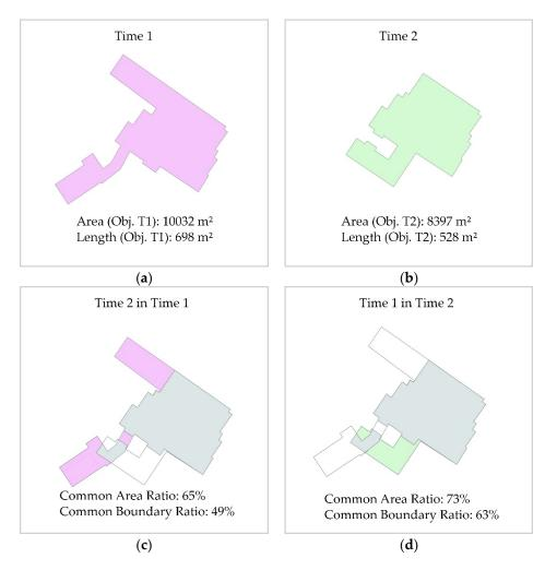
**Figure 3.** Examples of Common Area Ratio (*CAR*) and Common Boundary Ratio (*CBR*) for two footprints from different time points: (**a**) building at time 1; (**b**) building at time 2; (**c**) *CAR* and *CBR* of T1, T2; (**d**) *CAR* and *CBR* of T2, T1. Violet indicates the old area, green is the new area, and gray is the overlapping area.
