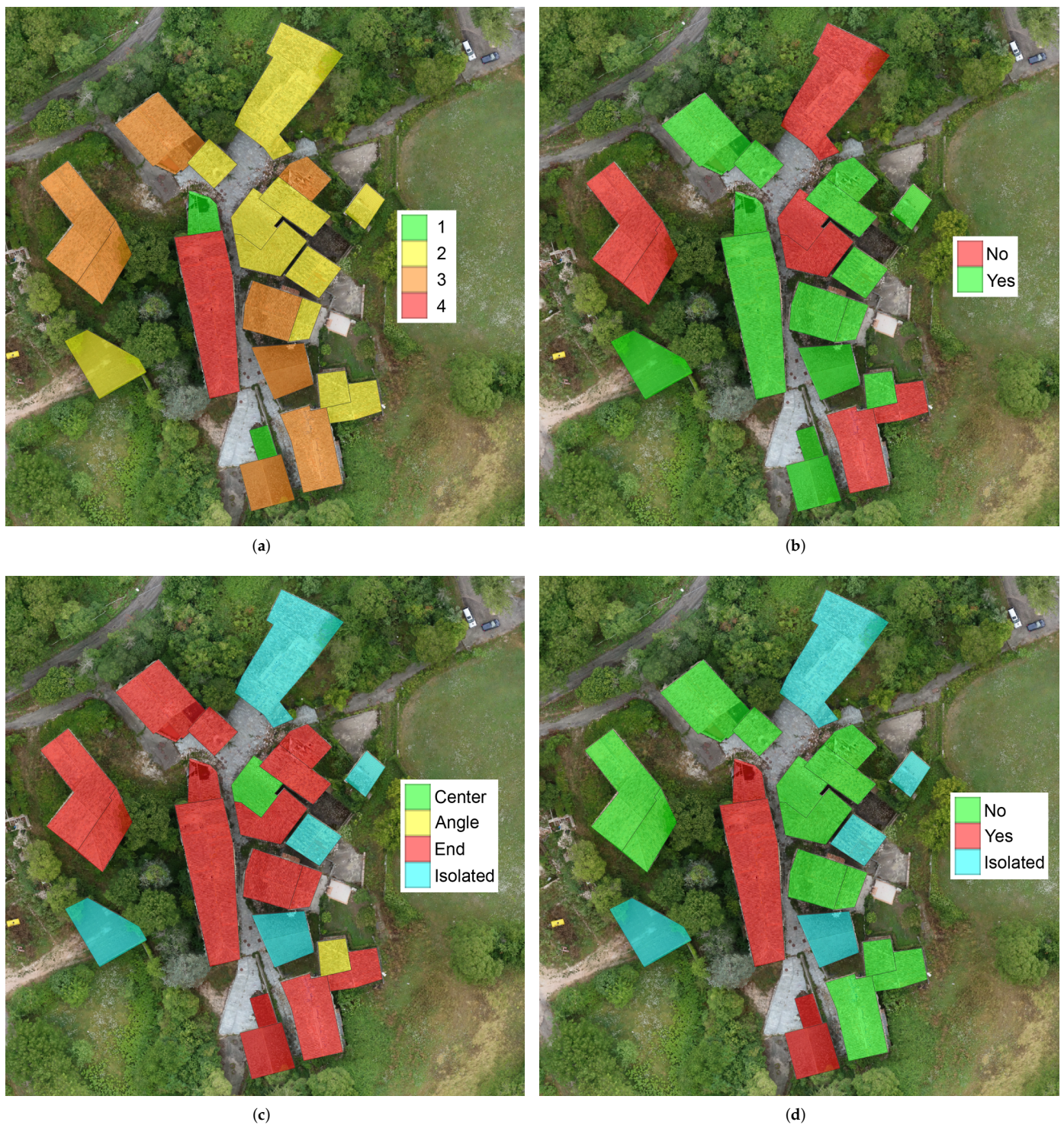
Figure 18. Thematic maps of the four extracted parameters of the buildings, shown in QGIS: (a) Number of floors (b) Shape regularity in plan (c) Planimetric location in the cluster (d) Presence of adjacent buildings with different height.
