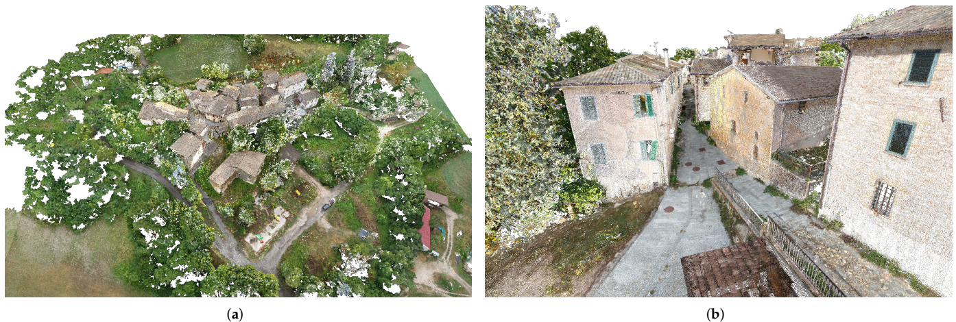
Figure 9. Unified point cloud: (a) Aerial view and (b) Street view.
