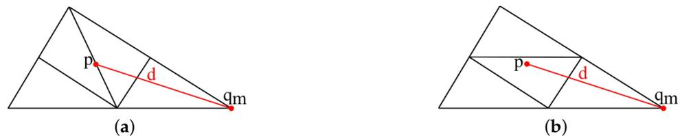
**Figure 10.** Two types of triangle 1 to 4 refinements with appropriate  $d$ . (a) 1:4 Longest-edge bisection, which is used in [26]. (b) 1:4 midpoint refinement which is a more common refinement.
