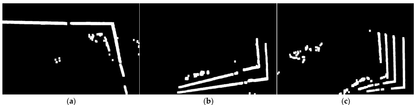
Figure 10. Binary masks for guiding neural restoration (office0); (a) Irregular corners and polyline deficiencies; (b) Multinested structures and parallel edge holes; (c) Complex geometric components and multilayer vertical edge holes.
