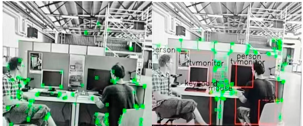
Figure 5. Comparison of feature point extraction performance between ORB-SLAM3 and the proposed method.
