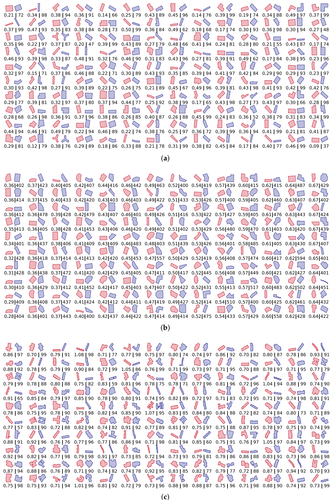
Figure 7. Shape pairs in distinct regions, with d_{TF} | d_{emb} values denoted below each pair. (a) Low d_{TF} low d_{emb} region: shape pairs satisfying d_{TF} < 0.5, d_{emb} < 100 . (b) Low d_{TF} high d_{emb} region: shape pairs satisfying d_{TF} < 0.7, d_{emb} > 400 . (c) High d_{TF} low d_{emb} region: shape pairs satisfying d_{TF} > 0.7, d_{emb} < 100 .
