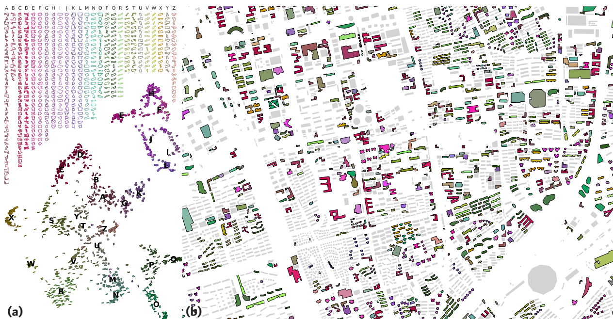
Figure 9. (a) Low-dimensional visualization of the embeddings for complex building shapes, together with representative instances from each cluster, reveals that recurring geometric patterns are consistently grouped in the embedding space. (b) When cluster labels are mapped back to geographic space for all building footprints, buildings assigned to the same cluster exhibit localized spatial aggregation in several areas.
