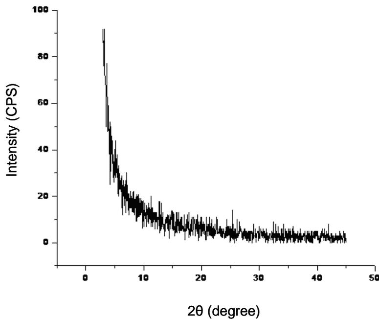
**Figure 3.** X-Ray Diffraction Analysis of the Carbon substrate.
