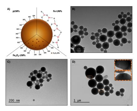
**Figure 6.** Schematic representation of the three types of lignin nanoparticles (LNPs) (**A**), and TEM images of (**B**) pLNPs, (**C**) Fe-LNPs and (**D**) Fe<sub>3</sub>O<sub>4</sub>-LNPs and magnification of the Fe<sub>3</sub>O<sub>4</sub> NPs inside the LNPs. (Reprinted with permission from [52]).
