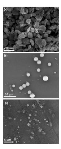
**Figure 7.** Scanning electron microcopy (SEM) images of **(a)** Zinc oxide nanoparticles **(b)** ligninnanoparticles organosolv and **(c)** lignin nanoparticles soda. (Reprinted with permission from [53].
