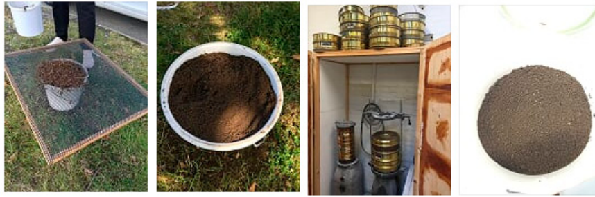
Supplementary Figure 4. Preparation of soil samples. Screening in a 10 mm mesh and a sieving tower with 2 mm screen.
