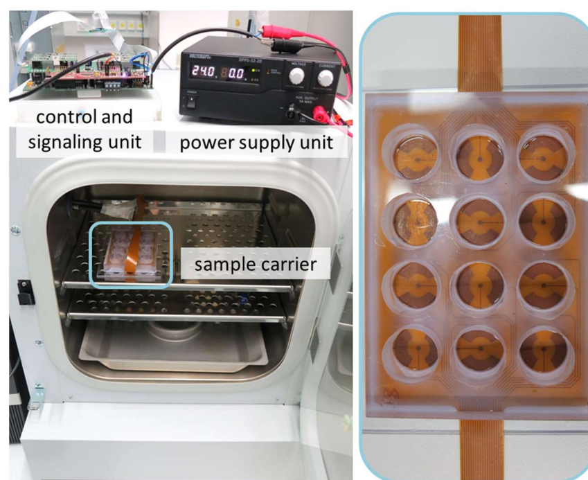
Figure 1. Overview of the stimulation device with control and signaling unit, sample carrier (detailed image; right) which is coupled to the electrodes and power supply unit.
