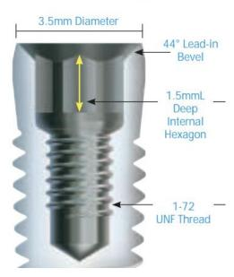
**Figure 5.** Zimmer Tapered Screw-Vent implant with the straight type of internal IAC. Reprinted with permission from the manufacturer.
