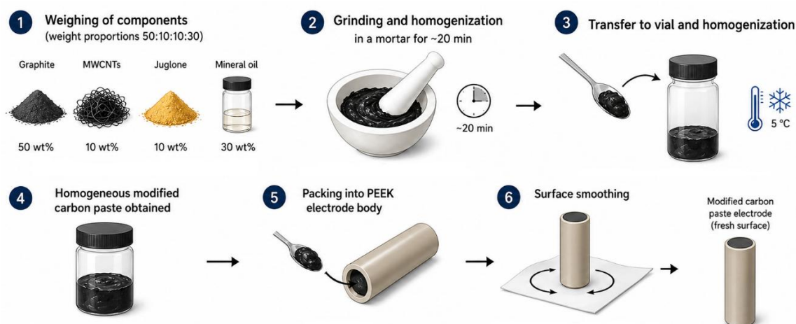
Figure 6. Visual presentation of JUG-MWCNTs/CP electrode preparation.
