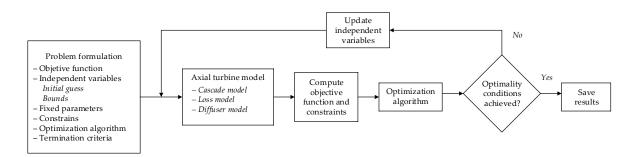
Figure 3. Axial turbine optimization strategy flow diagram.
