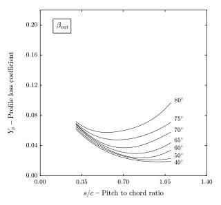
Figure A1. Profile loss of reaction blades (axial entry blades).
