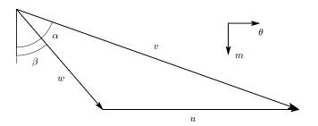
Figure 2. Velocity triangle showing the notation and conventions used in this work.
