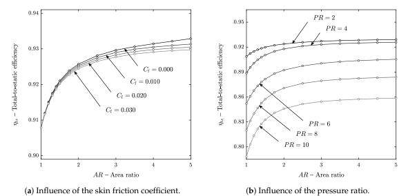
**Figure 5.** Total-to-static isentropic efficiency as a function of the diffuser area ratio and (**a**) skin friction coefficient or (**b**) pressure ratio.
