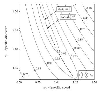
Figure 7. Balje diagram of the reference case.
