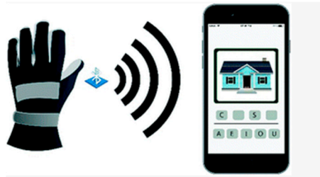
Figure 3. Design of an electronic glove for teaching vowels for deaf children. In [31].
