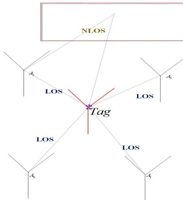
**Figure 4.** NLOS problem: In the absence of LOS in TOF-based ranging between MN and AP, the estimated range is larger than the true distance.
