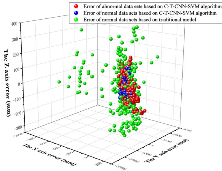
**Figure 17.** Comparison of 3D (X, Y, Z) accuracy of C-T-CNN-SVM and traditional algorithms.
