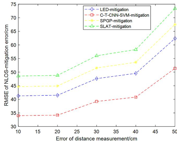
**Figure 9.** Comparison of NLOS mitigation performance between the proposed and other state-of-the-art algorithms.
