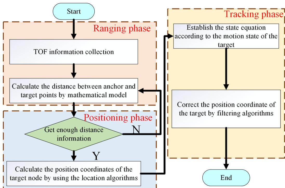
Figure 1. Overall model of accurate UWB localization.
