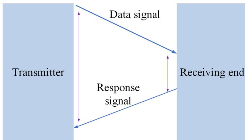
Figure 3. Schematic diagram of TOF ranging method.
