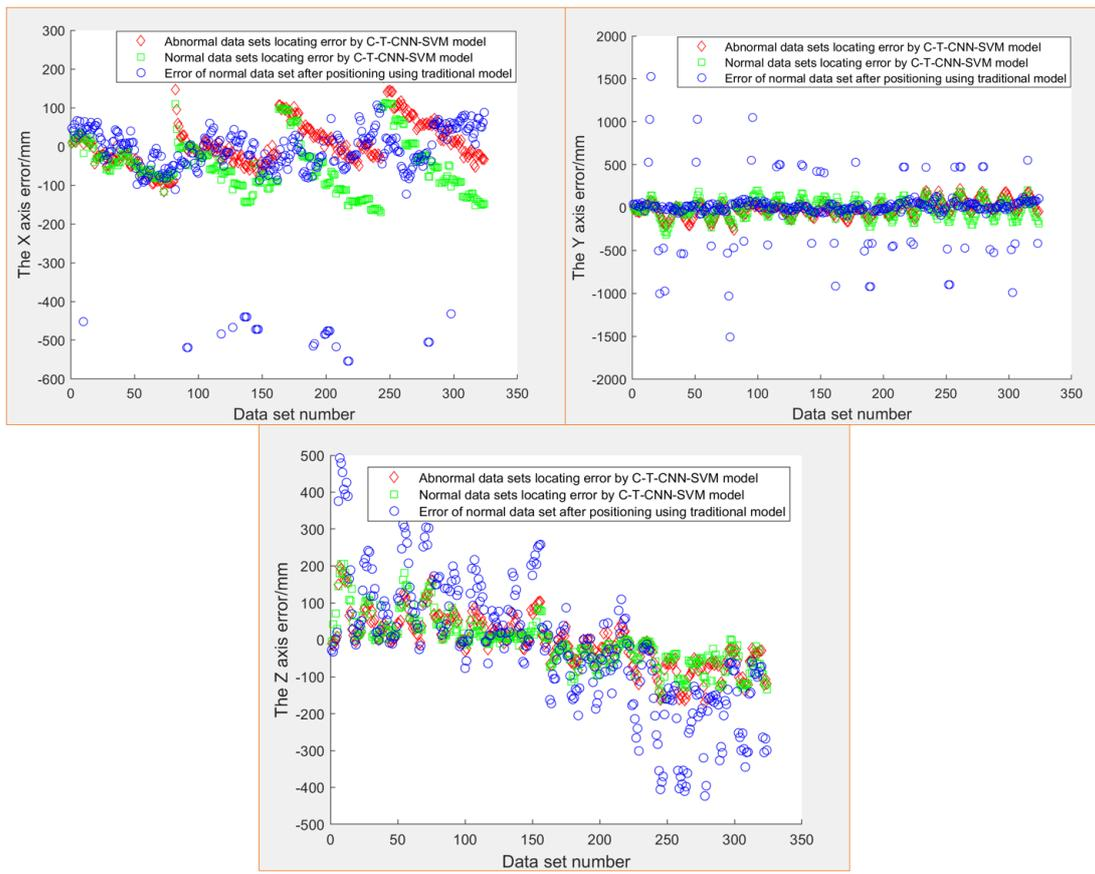
Figure 10. 1D accuracy of abnormal data sets based on C-T-CNN-SVM algorithm.
