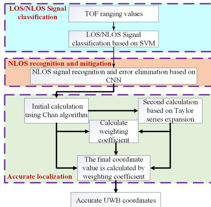
Figure 6. General flow chart of C-T-CNN-SVM algorithm.
