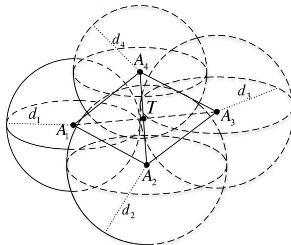
Figure 5. Traditional quadrilateral location algorithm.
