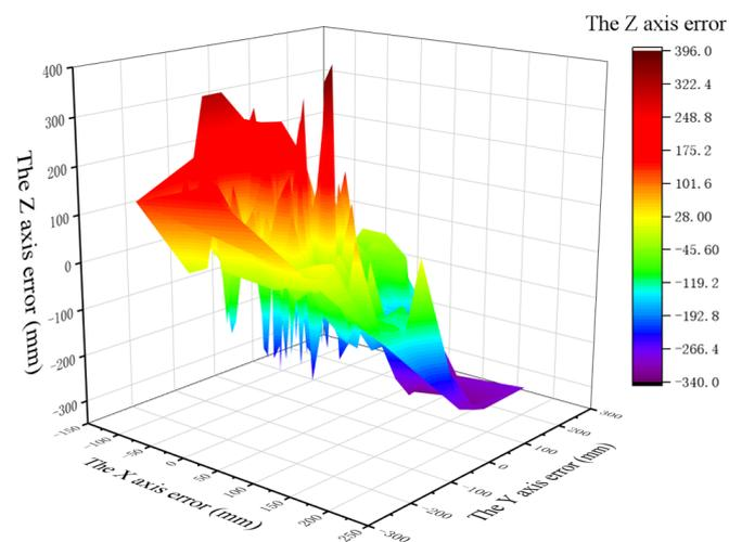
Figure 16. 3D (X, Y, Z) accuracy of normal data sets based on traditional model.
