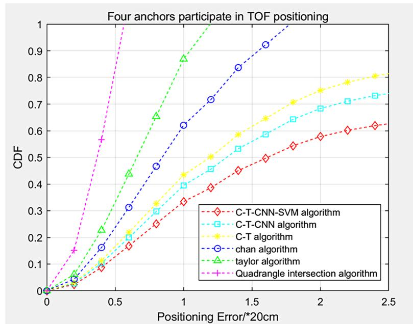
Figure 18. Relation curve between CDF distribution and location error of each algorithm.
