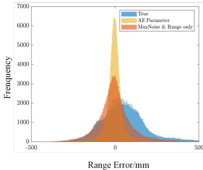
**Figure 8.** Effect of CNN-based NLOS error mitigation.
