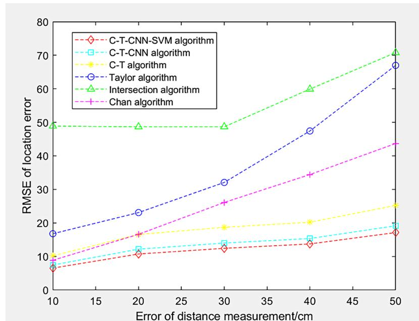
Figure 19. Relation curve between root-mean-square distribution and location error of each algorithm.
