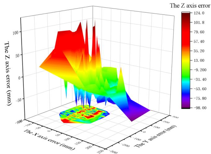
Figure 15. 3D (X, Y, Z) accuracy of normal data sets based on C-T-CNN-SVM algorithm.
