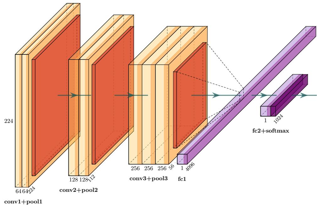
**Figure 7.** CNN structure for NLOS signal recognition.
