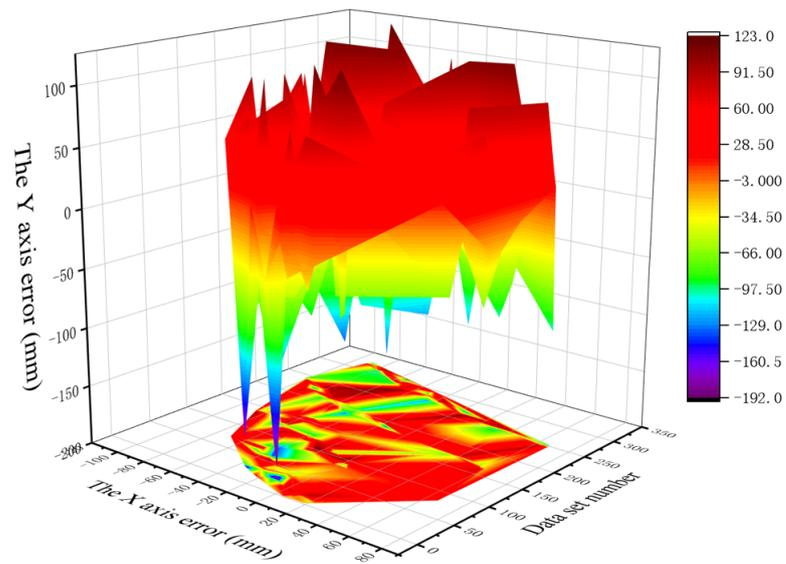
Figure 12. 2D (X, Y) accuracy of normal data sets based on C-T-CNN-SVM algorithm.
