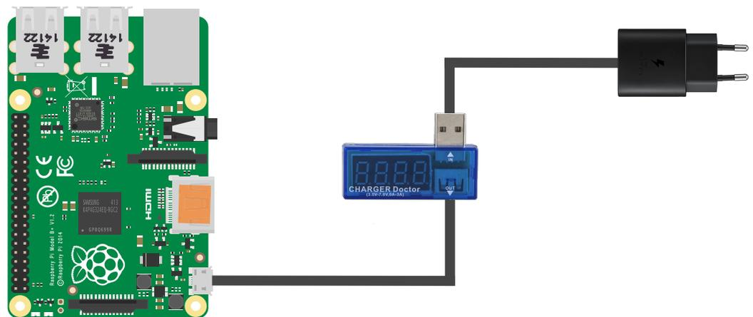
**Figure 12.** Experimental setup for the energy analysis. The dedicated energy measurement hardware sits on the connection between the Raspberry Pi and the power outlet.
