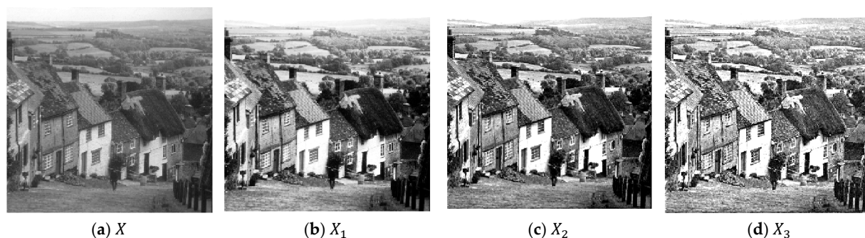
Figure 16. (a) The original image ‘Goldhill512.bmp’ 512 × 512, (b) the histogram equalization, and the images enhanced by (c) the 0.85-rooting and (d) the negative 0.85-rooting.
