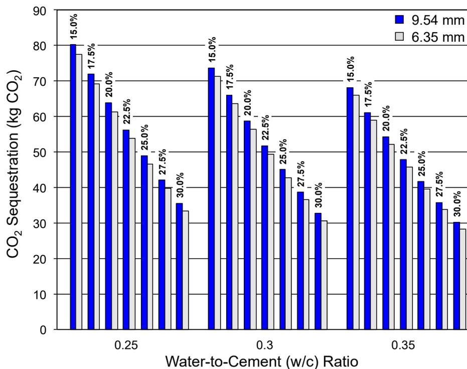
**Figure 3.** CO<sub>2</sub> sequestration potential for 1 m<sup>3</sup> of pervious concrete. Design porosity of each mixture is indicated above its respective column. Aggregate size is differentiated by color.
