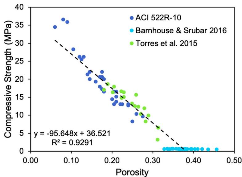
**Figure 1.** Relationship between compressive strength and porosity [4,10,38].
