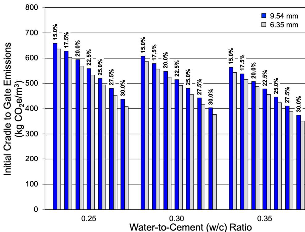
**Figure 2.** Initial cradle-to-gate CO<sub>2</sub>e emissions of pervious concrete mixtures designed according to the NRMCA design methodology [35,36]. Design porosity of each mixture is indicated above its respective column. Aggregate size is differentiated by color.
