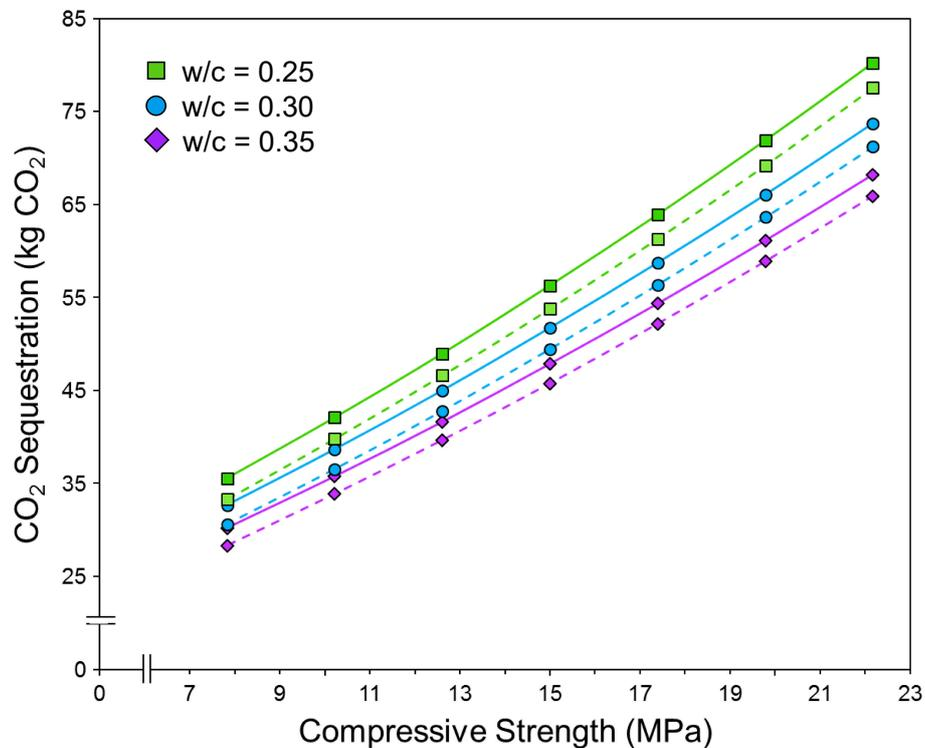
**Figure 4.** Effect of compressive strength on the CO<sub>2</sub> sequestration potential of 1 m<sup>3</sup> of pervious concrete with varying water-to-cement (w/c) ratios and both 9.35 mm (—) and 6.35 mm (- - -) aggregate.
