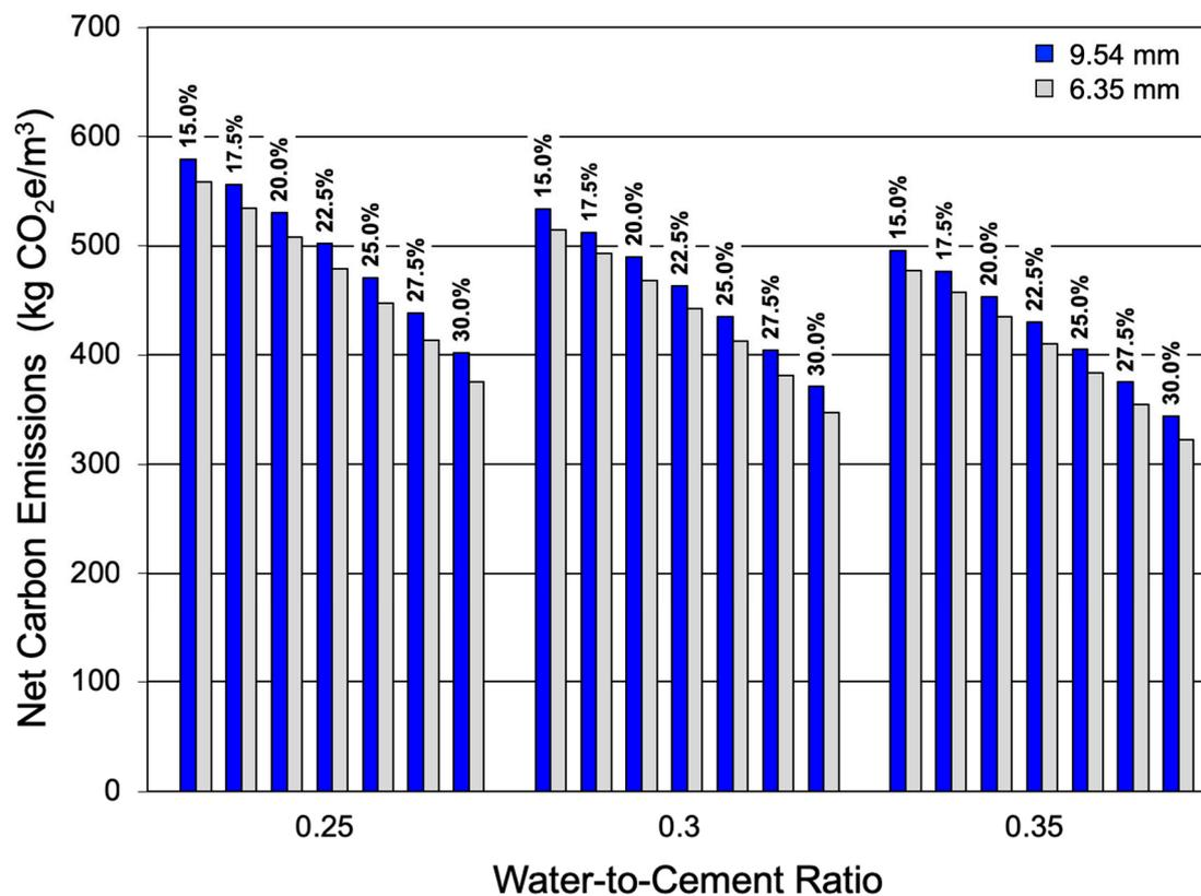
Figure 6. Net CO<sub>2</sub>e emissions of 1 m<sup>3</sup> of pervious concrete. Design porosity of each mixture is indicated above its respective column. Aggregate size is differentiated by color.
