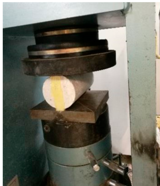
Figure 10. Laboratory configuration for the splitting strength test.
