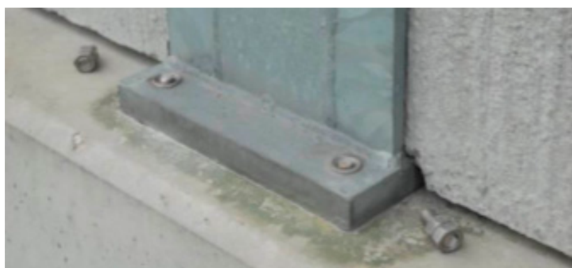
Figure 6. Fatigue failure of threaded bolts used for fastening of NB steel posts.
