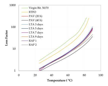
Figure 6. Loss factor versus temperature curve.
