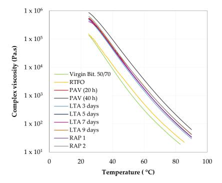
Figure 8. Complex viscosity curve.
