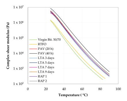
Figure 7. Isochronal plots of the complex shear modulus (G\*).
