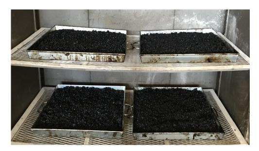
Figure 2. Loose asphalt mixture oven ageing.
