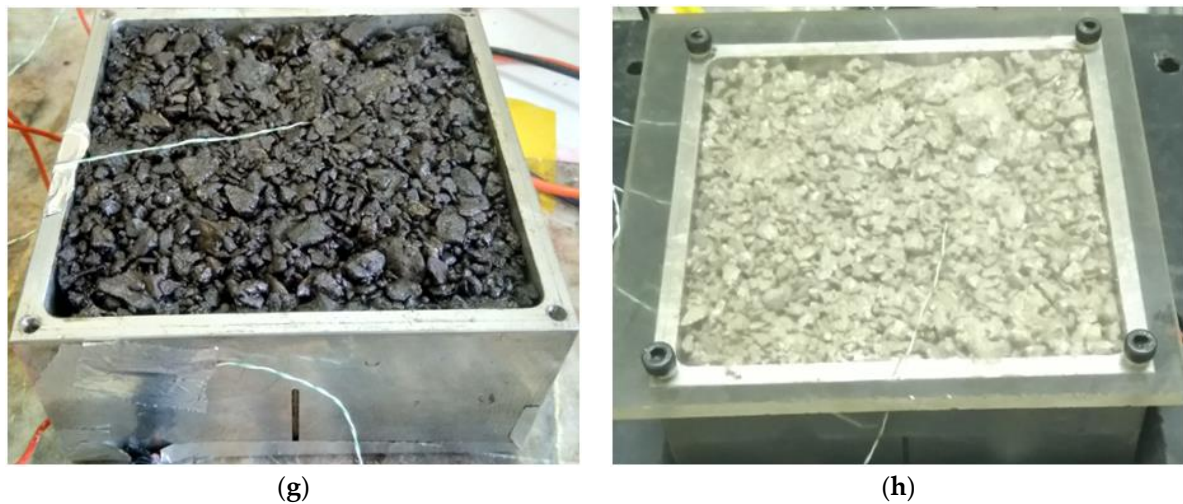
Figure 2. Steps involved in the preparation of binders and asphalt mixtures for thermal analysis. (a) \text{TiO}_2 being mixed with dry aggregates. (b) Binder poured into the \text{TiO}_2 blended aggregates. (c) Placement of a silicon heater at the base of the heat sink. (d) Heat sink inside the fiber block insulation, with installed thermocouples and heater. (e) White pigmented ( \text{TiO}_2 ) clear binder poured into a container. (f) \text{TiO}_2 -modified CB under experimentation. (g) Conventional asphalt inside the large heat sink, with installed thermocouples and heater. (h) White pigmented asphalt mixture before the start of the test.
