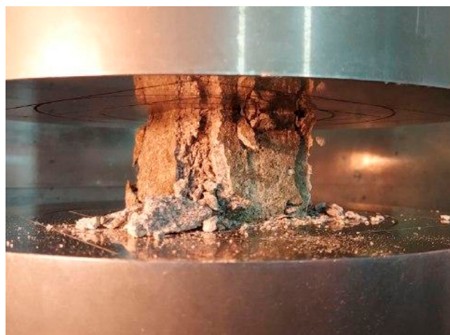
Figure 2. Compression test of a 100 \times 100 \times 100 mm cube specimen.
