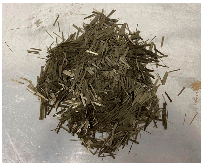
Figure 1. Chopped pieces of complex threads made of basalt fiber.
