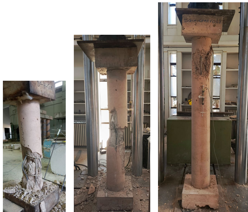
Figure 9. Failure modes of heated control specimens (H-80-Control, H-120-Control, and H-150-Control).
