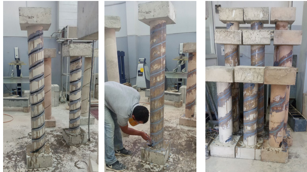
Figure 6. Installing of CFRP rope.
