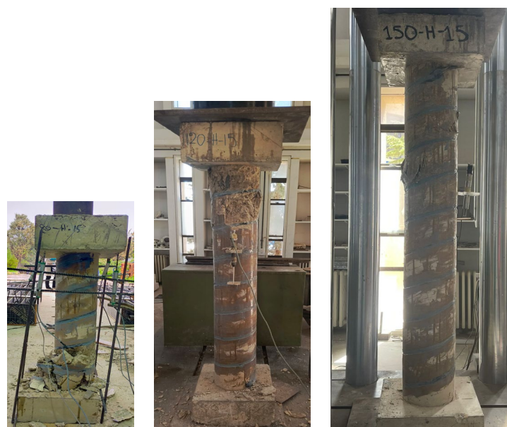
Figure 11. Failure modes of repaired heated column with rope at 150 mm spacing (H-80-R15, H-120-R15, and H-150-R15).
