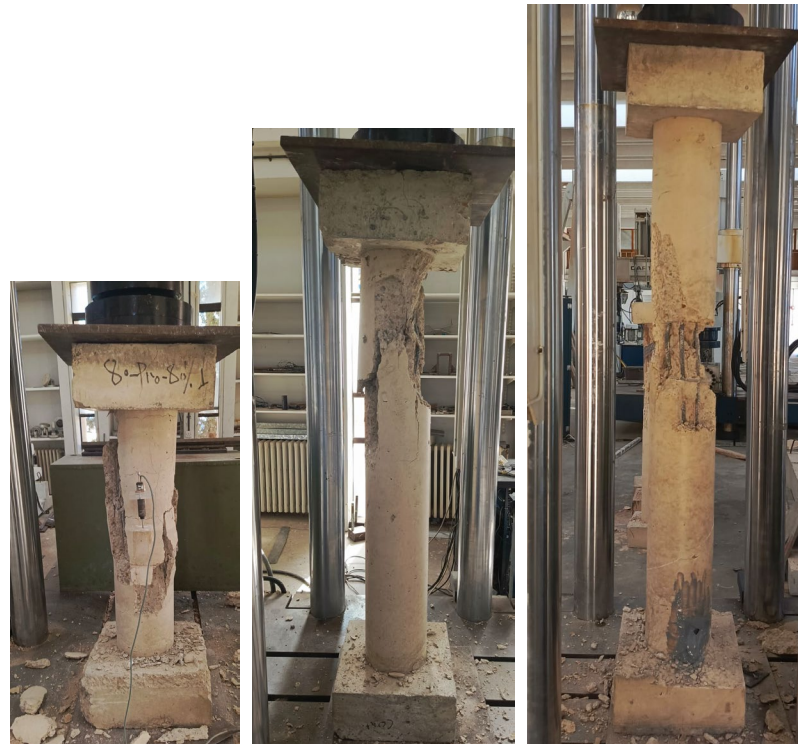
Figure 8. Failure modes of unheated control specimens (UH-80-Control, UH-120-Control, and UH-150-Control).
