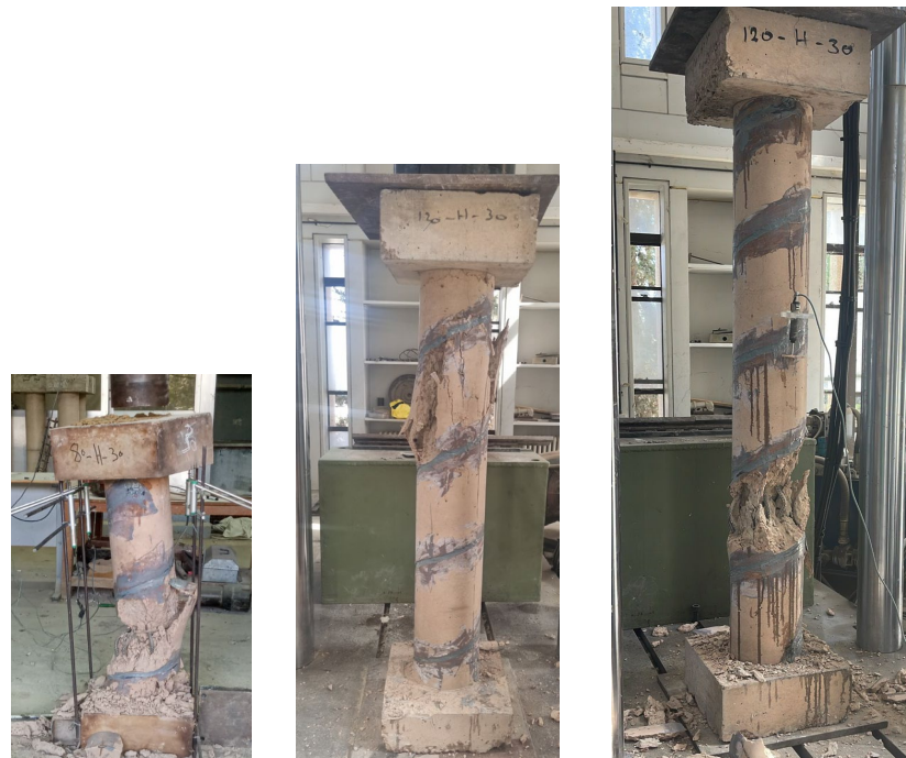
Figure 10. Failure modes of repaired heated column with rope at 300 mm spacing (H-80-R30, H-120-R30, and H-150-R30).
