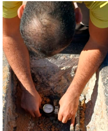
Figure 11. Installation of strain gauges.
