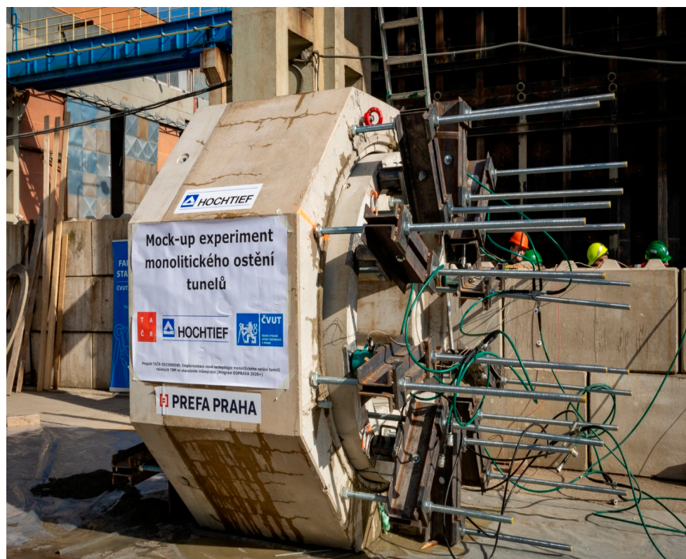
Figure 8. Specimen fitted with hydraulic cylinders.
