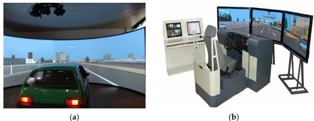
Figure 2. Driving simulator for testing: true car cab (a), self-built cockpit (b).
