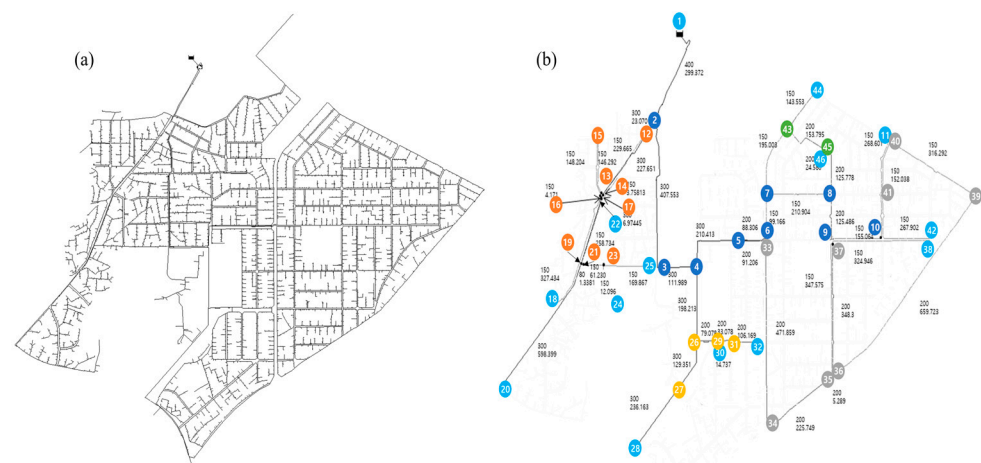
Figure 2. QGIS-based maps of the water distribution network in Y District, D Metropolitan City: (a) original network; (b) skeletonized network. Colored dots and number labels indicate network nodes and node IDs, respectively.
