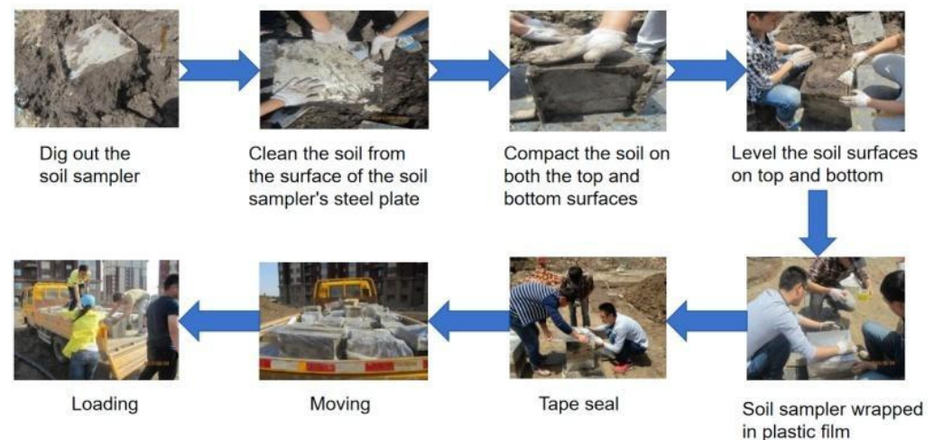
Figure 8. The manufacturing and transportation process of soil samplers.
