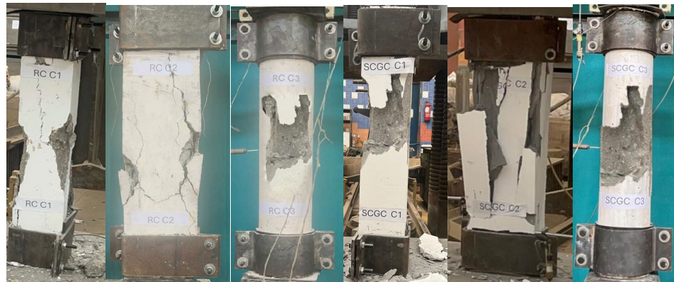
Figure 4. Observed failure modes of Groups G1 (RC columns) and G2 (SCGC columns).
