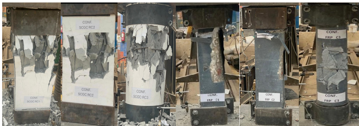
Figure 5. Observed failure modes of Group G3 (SCGC-jacketed confined columns, CONF. SCGC) and Group G4 (CFRP-wrapped confined columns, CONF. FRP).
