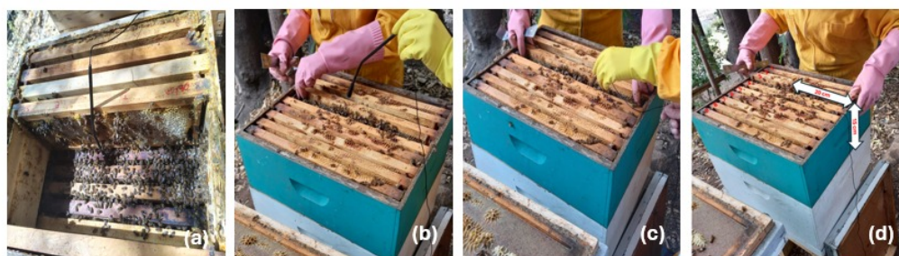
Figure 1. Test with different position between frames (a); hive without queen (b); Installation of the microphone between frames most representative of the worker population (c); and distance of microphone between brood chamber and honey super (d).
