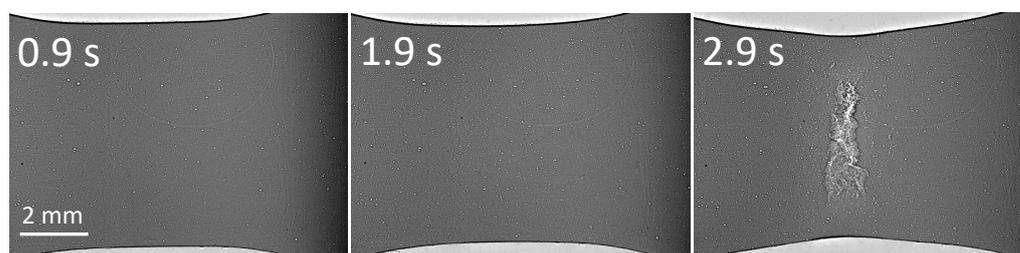
**Figure 5.** X-ray images of Scalmetalloy specimen (printed 0° flat) under tension in quasi-static UTM. Image series captured by Photron SA-Z high speed camera at 10 kHz frame rate and a resolution of  $1024 \times 1024$  pixels. From left to right, different timestamps capturing the formation of voids to fracture. White contrast in these radiographs represent high intensity X-rays. The aspect ratio of the images are adjusted for illustration purposes.
