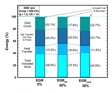
**Figure 19.** The partition of the fuel exergy for three cases: 0% EGR, 30% EGR adiabatic, and 30% EGR cooled.
