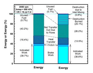
Figure 2. Partition of energy and exergy for case 1.
