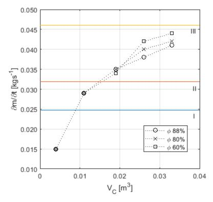
Figure 6. Relation of volume of product to required refrigerant flow.
