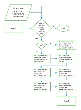
**Figure 2.** Stage 1 of the algorithm. The internal air analysis described in Equations (1)–(17).
