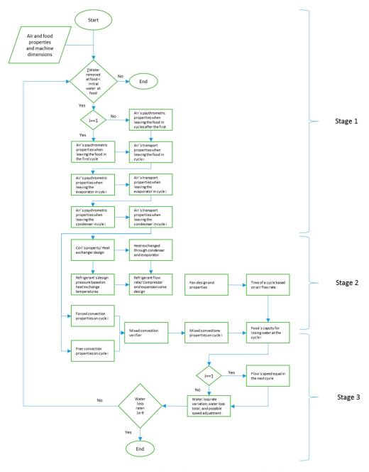
Figure 5. Heat pump dryer design optimization algorithm
