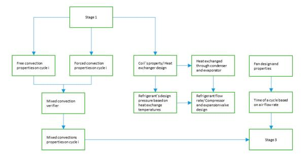
**Figure 3.** Stage 2 of algorithm. Heat flow analysis between components, air and food. Component design derived from Equations (18)–(24).
