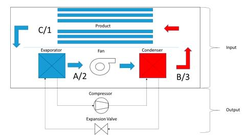
**Figure 1.** Scheme of a specific prototype of a heat pump food dryer tested for this algorithm where the thin line represents the refrigerant circuit while the thick arrows represent the airflow circuit.
