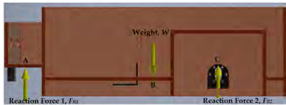
Figure 3. Free-body diagram of the lawnmower.
