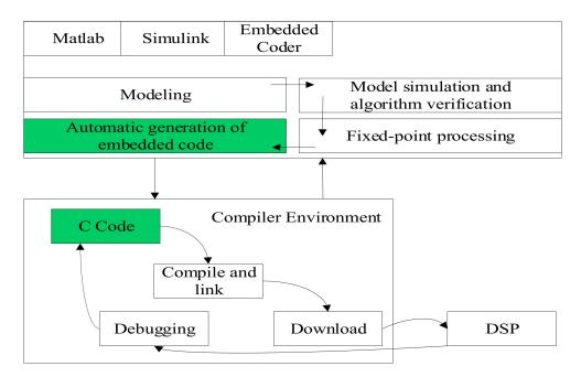
Figure 4. The embedded code automatic generation process of DSP.
