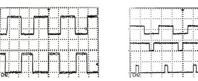
(a) Peak-peak value 424 mV Average value 132 mV Cycle 272.8 us Frequency 3.666 kHz
