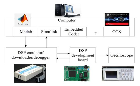
**Figure 6.** The composition and schematic diagram of the experimental software and hardware platform.
