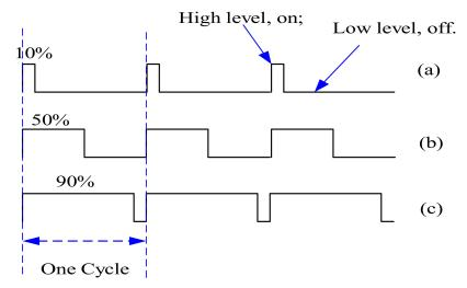
**Figure 5.** The technology of PWM. (a) the duty cycle is 10%; (b) the duty cycle is 50%; (c) the duty cycle is 90%.
