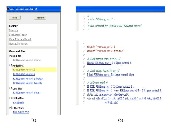
**Figure 7.** Code generation report and its generated files. (a) code generation report; (b) generated C file.
