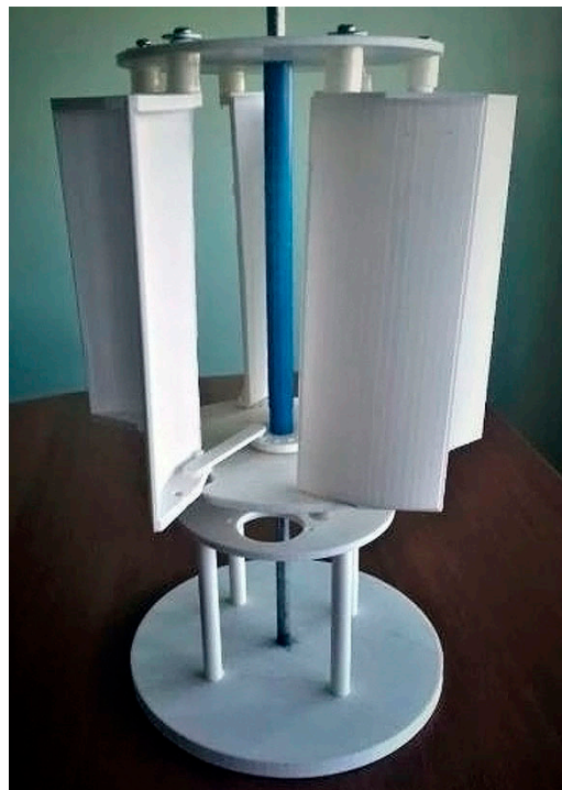
Figure 14. Implemented laboratory 3D model of a wind turbine.
