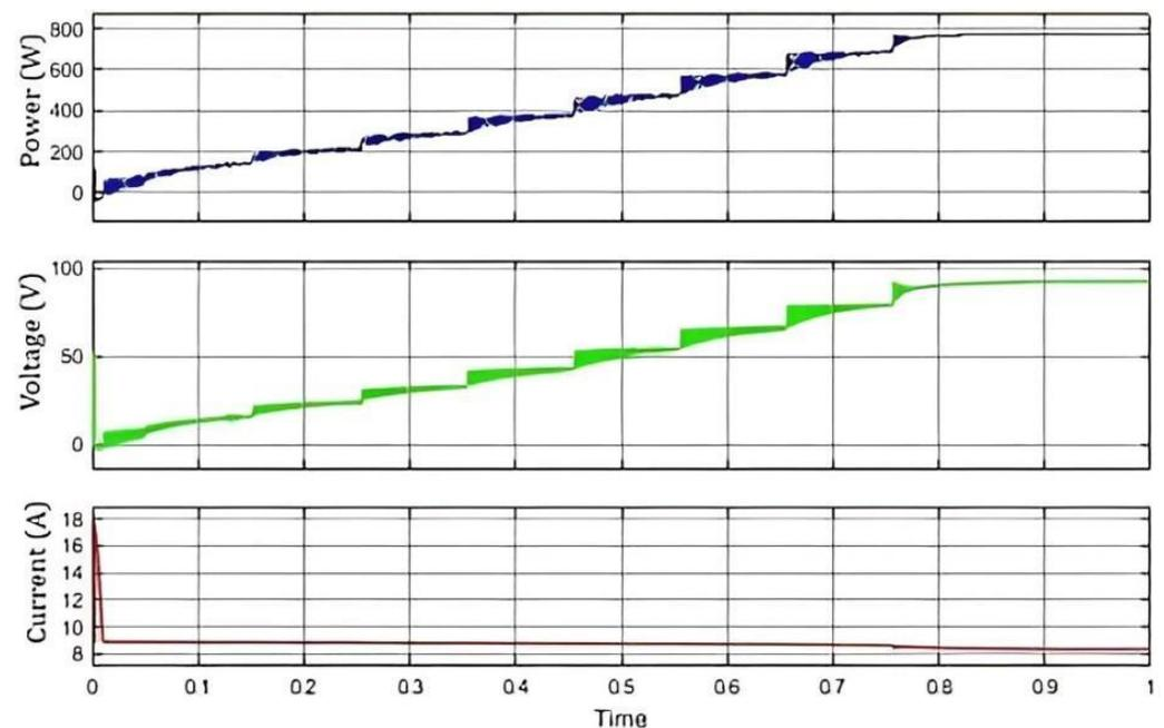
**Figure 6.** Case 1: power, voltage, and current versus time for the P&O MPPT method.
