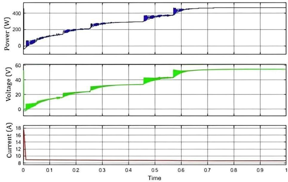
Figure 9. Case 2: power, voltage, and current versus time for the P&O MPPT method.
