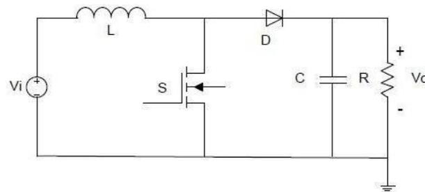
**Figure 1.** Boost converter circuit schematic.
