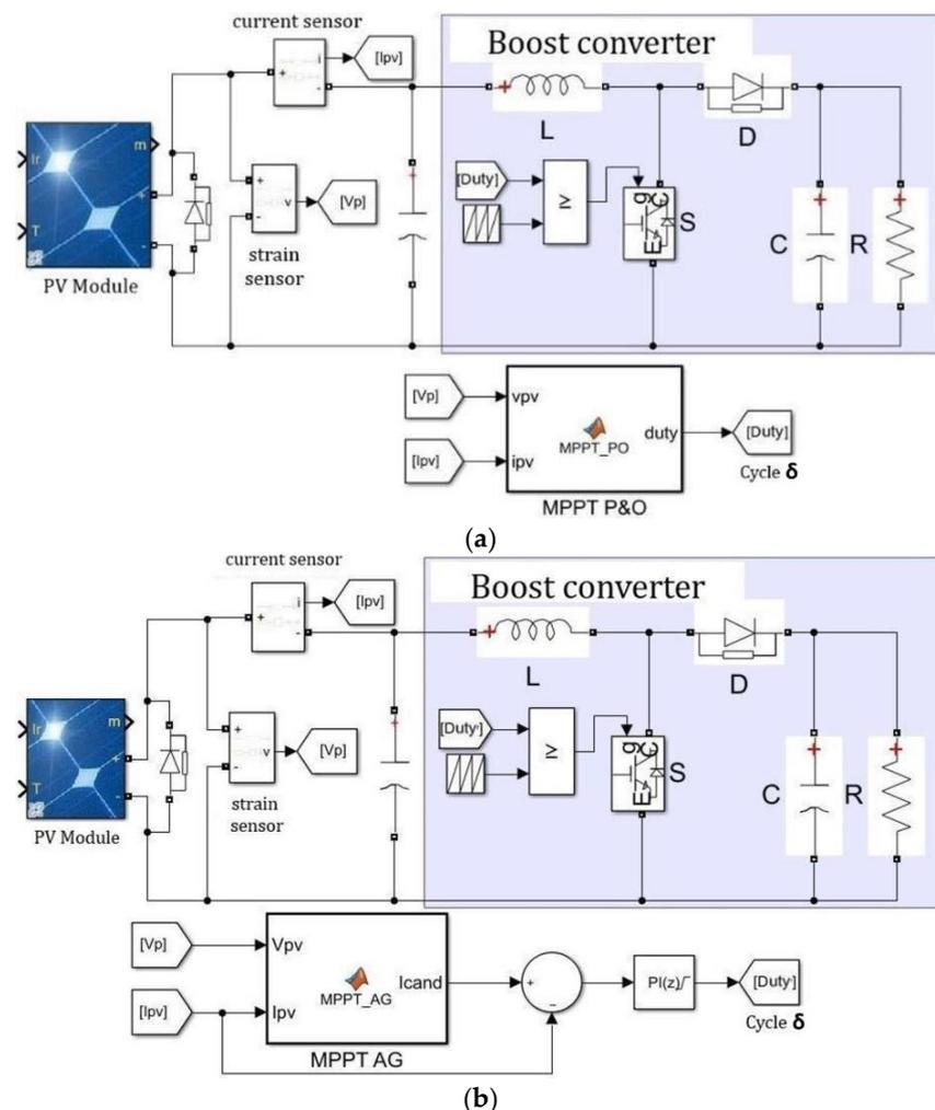
**Figure 5.** MPPT controller configurations for the duty cycle to the boost converters, depicting (a) the P&O method and (b) the GA-based method.
