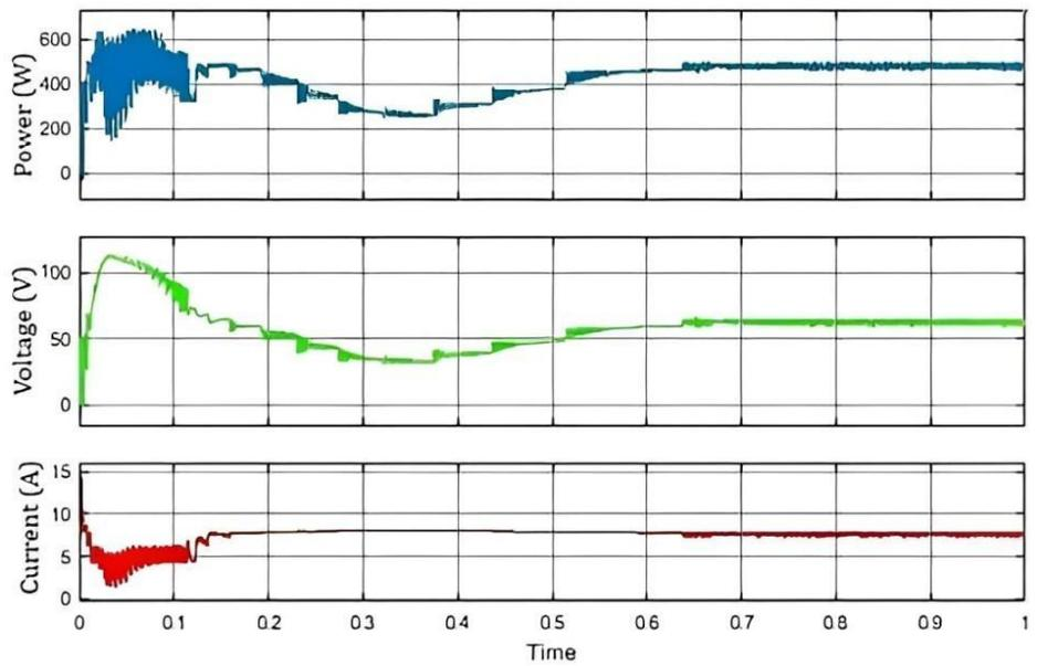
Figure 13. Case 3: power, voltage, and current versus time for the GA-based MPPT technique.
