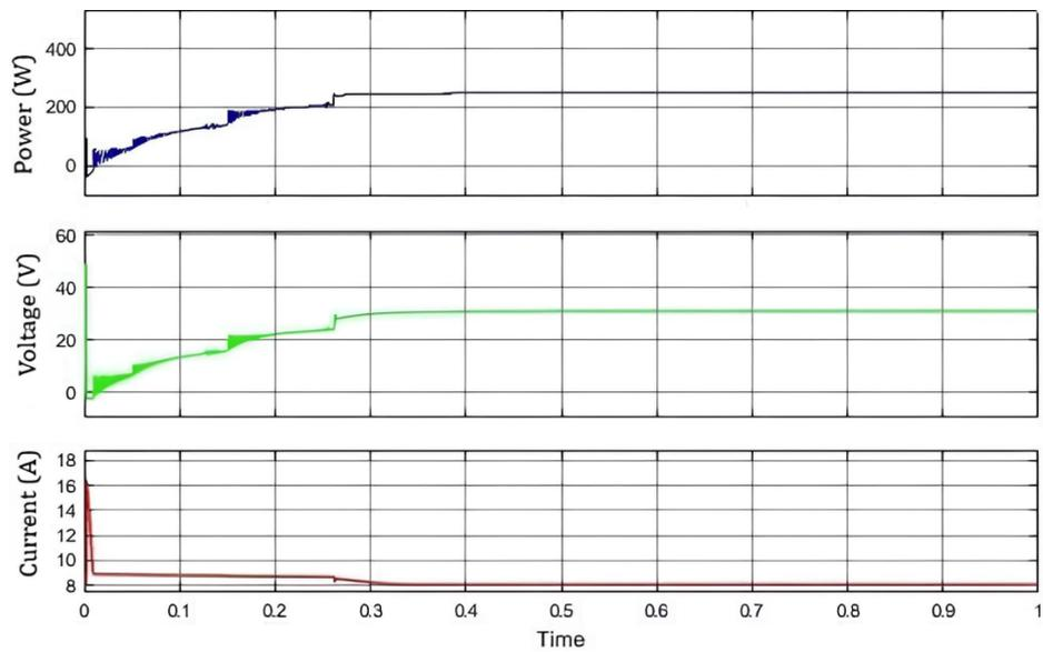
Figure 12. Case 3: power, voltage, and current versus time for the P&O MPPT method.
