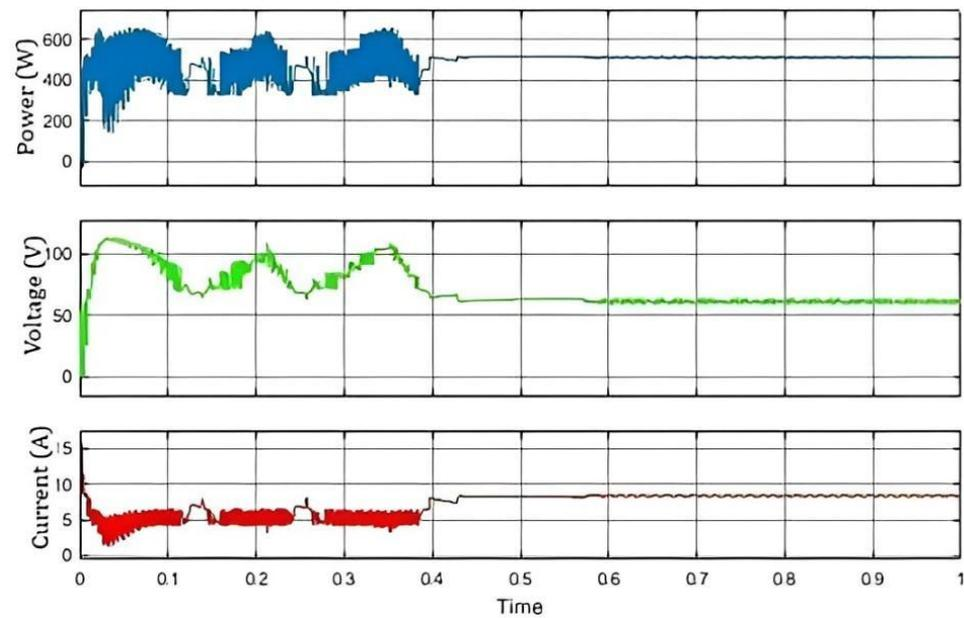
Figure 10. Case 2: power, voltage, and current versus time for the GA-based MPPT technique.
