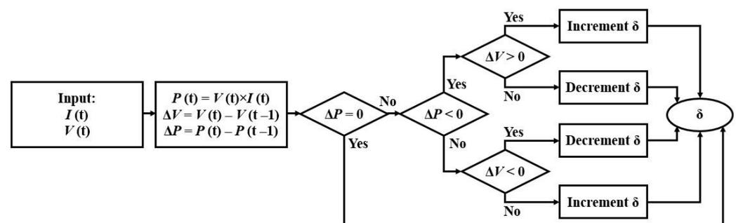
Figure 3. Flowchart of the P&O MPPT method.
