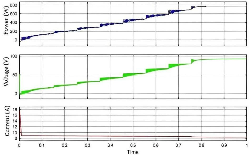
Figure 7. Case 1: power, voltage, and current versus time for the GA-based MPPT technique.
