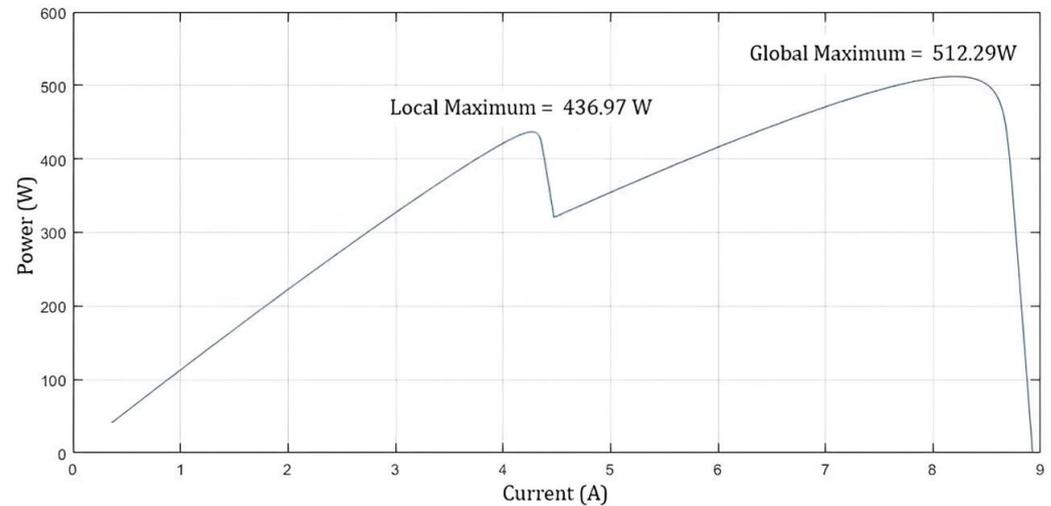
Figure 8. Case 2: power versus current characteristic curve.
