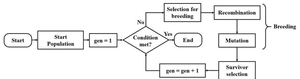
**Figure 4.** Typical GA-based MPPT flowchart.
