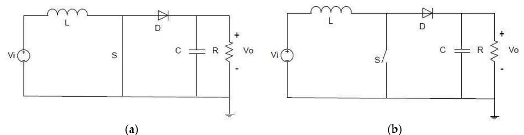
**Figure 2.** Simplified circuit schematic of the boost converter, showcasing configurations with (a) the switch closed and the diode open, and (b) the switch open and the diode closed.
