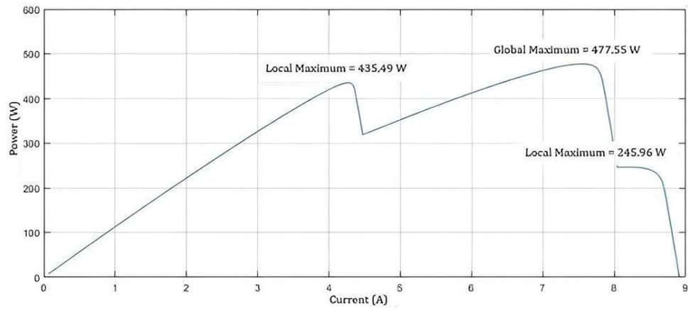
Figure 11. Case 3: power versus current characteristic curve.
