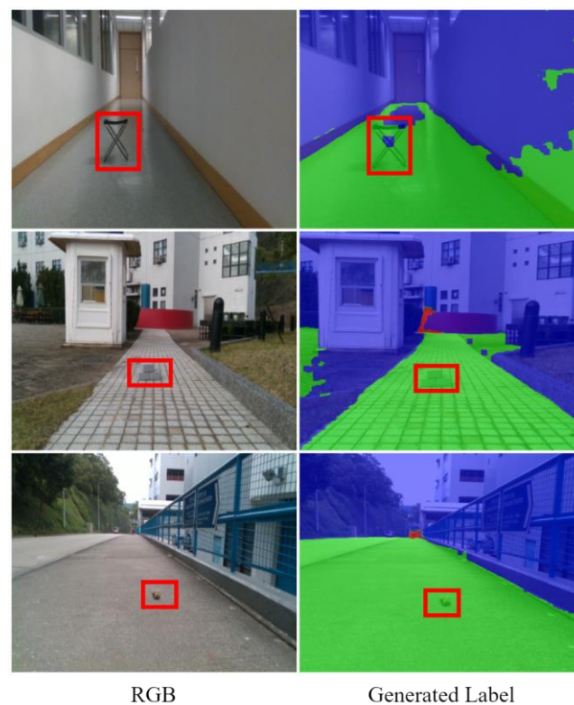
Figure 13. Some cases of failure when applying our ALS framework. The red boxes indicate the location of the road anomalies in the images. The red, green, and blue colors represent the obstacle, drivable area and background, respectively
