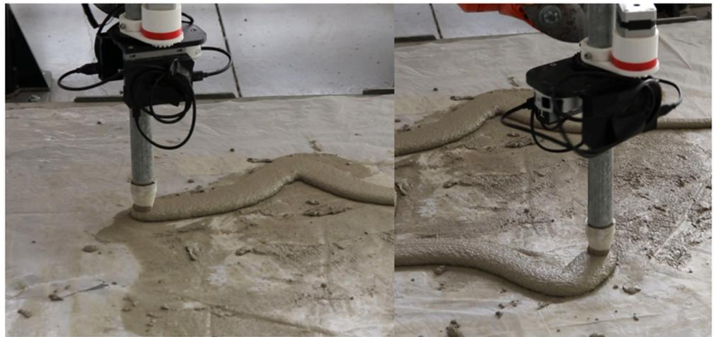
**Figure 23.** Automatic self-alignment of the camera with the extrusion by the rotary system.
