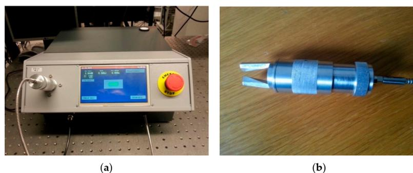
**Figure 2.** (a) The complete blue laser source with a touchscreen, which allows for setting the treatment parameters. A foot pedal is connected at the bottom (black cable). (b) The handpiece (applicator) at the end of the fiber. This applicator is inserted into the power meter in the photo on the left.
