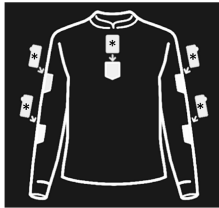
Figure 1. Visual description of IMU sensors (marked with asterisks) placement in the Niurion ® shirt.
