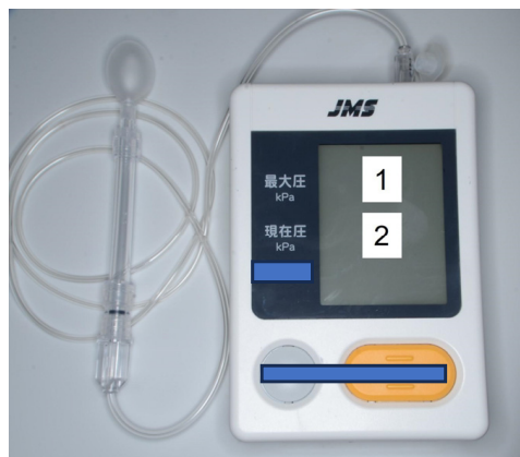
Figure 1. Tongue-pressure-measuring instrument equipped with a balloon probe. Maximum tongue pressure (kPa) is displayed in box 1, and current tongue pressure (kPa) is displayed in box 2.
