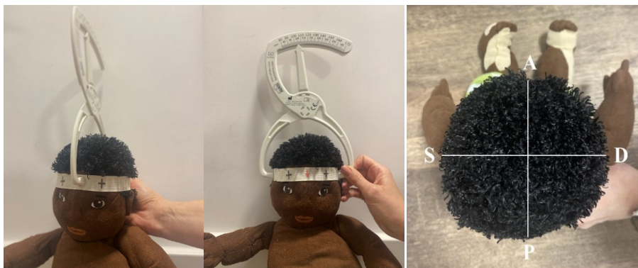
Figure 3. Proportion Measurement Schema. The schematic illustrates the two distances measured: (1) the widest point of the head, taken with the craniometer parallel to the face (SD measurement, sinistra/dextra) and (2) the longest point of the head, taken with the craniometer perpendicular to the face (AP measurement, anterior/posterior).
