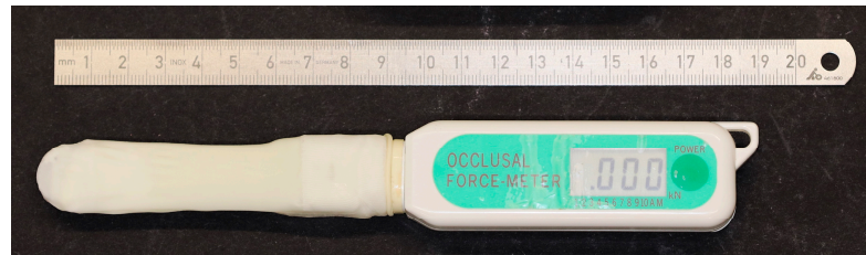
Figure 1. The Occlusal Force Meter GM 10 (OFM) for measuring the bite force in newtons with a hygienic protective cover.
