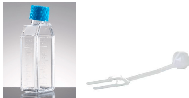
Figure 1. Group 1 (G1): 50 mL Corning® CellBIND® Surface Cell Culture Flask (Corning Incorporated—Life Sciences, Durham, NC, USA) with Böhnke donor corneal holder® (Bausch & Lomb Incorporated, Eppelheim, Germany).
