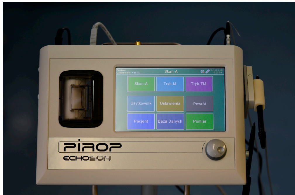
Figure 1. The PIROP-G ultrasound-based system (ECHOSON S.A., Puławy, Poland) used for non-invasive measurement of peri-implant soft tissue thickness in the present study.
