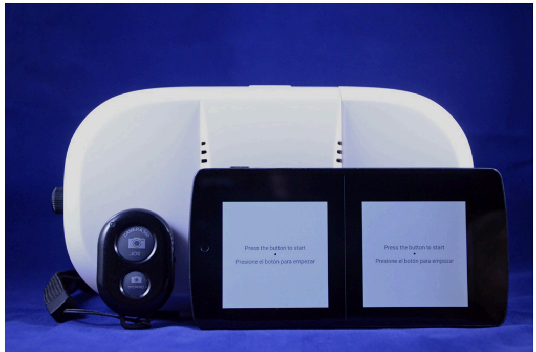
Figure 3. Mobile virtual perimetry model consisting of a smartphone, virtual reality headset, and remote [22].
