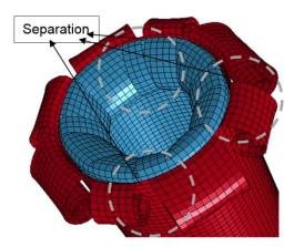
**Figure 24.** Effect of stacking sequence of  $[0]_{12}$  configuration on petal formation of FEM crushed morphologies using DFAILM [59].
