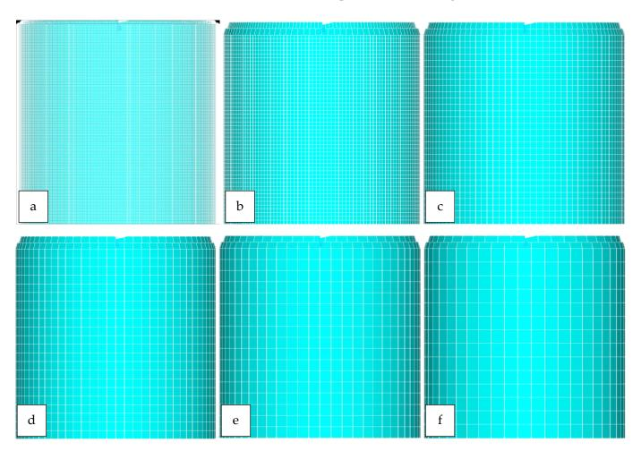
computable costs is also relatively important. Six different element sizes were modelled with 5.5, 4.5, 3.5, 2.5, 1.5, 0.5 mm quad elements (see Figure 6).
