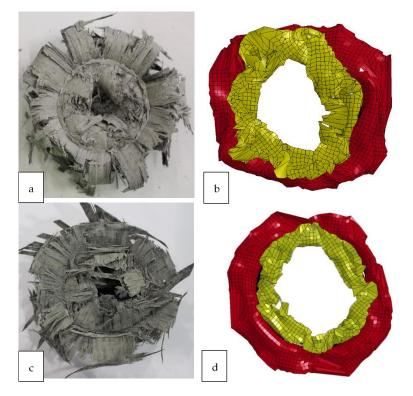
**Figure 27.** Plane view morphologies, experimental and numerical comparison, (**a**) crushed under quasi-static experimental, (**b**) crushed under quasi-static numerical, (**c**) crushed under impact loading experimental, (**d**) crushed under impact loading numerical [63,65].
