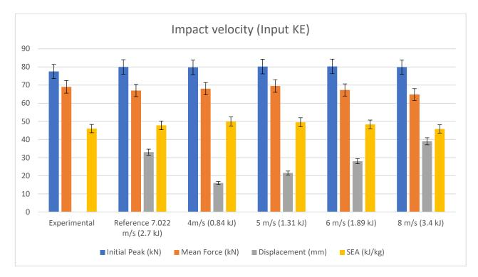
energy absorption, which indicates the energy absorption per crushed mass, is within 4% of the reference model. The mean crushing force is slightly affected, although the highest difference from the reference model is 3.5%.
