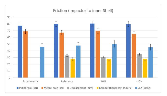
Figure 20. Impactor to inner-shell friction coefficient comparison [66].
