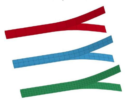
Figure 17. Tiebreak contact element size test [66].
