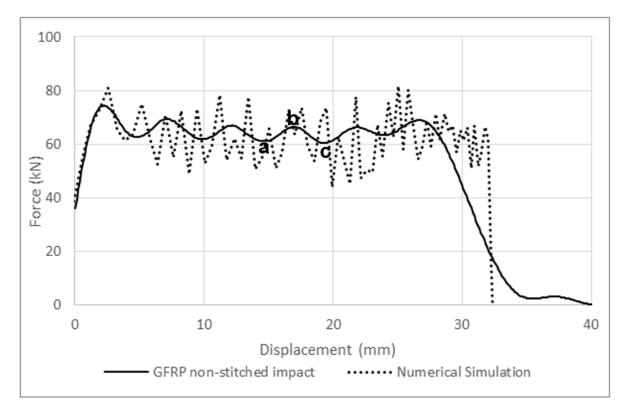
**Figure 26.** Force–displacement characteristic experimental and numerical comparison [66], (a–b) increase in load and(b–c) decrease in load.
