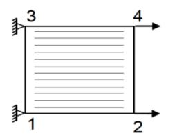
Figure 1. Single 4-node shell element under tension [51].
