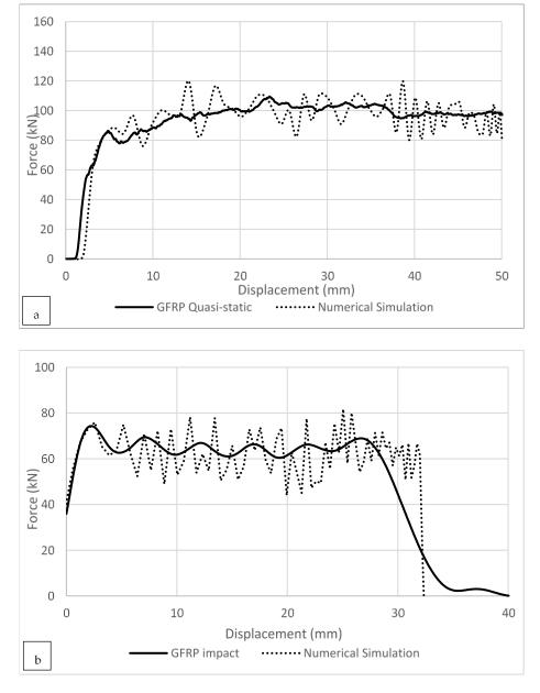
Figure 28. Force-displacement characteristic experimental and numerical comparison [66].
