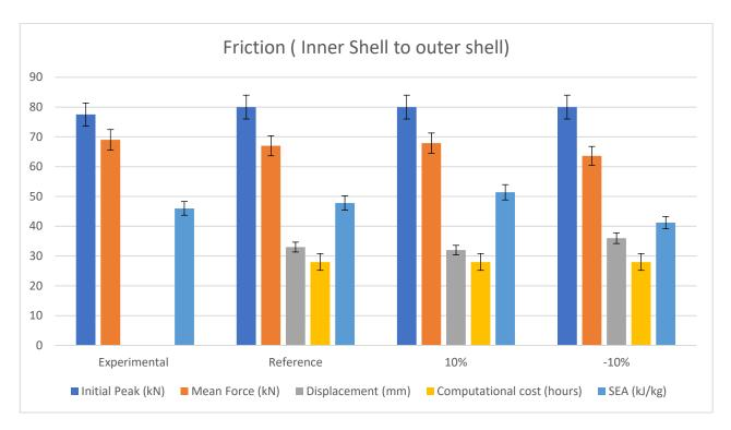
Figure 21. Inner-shell to outer-shell friction coefficient comparison [66].
